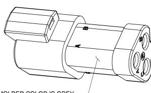
RECEPTACLE, 3 PIN, AT SERIES, SOLID REAR SEAL, END CAP
